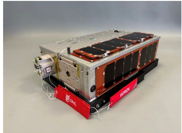
WREN-1 showing two optics openings, S-band antenna, OWL, stowed UHF antenna and solar panels
